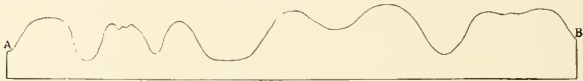
FIG. 14. Profile of surface between points "A" and "B", PLATE II, showing irregular topography occasioned by small valleys.
